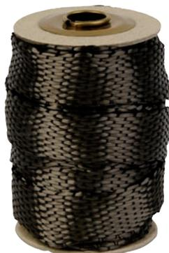
unidirectionally woven carbonfibre elastic stockinette, approx. 20 - 50 mm stretchable, for conical or undulated models, suitable for axial-reinforcements PU = 5 m
