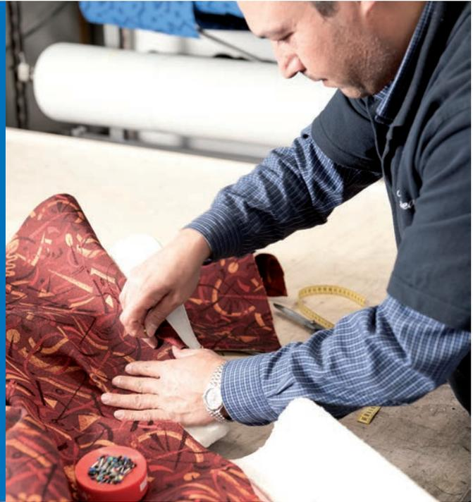
The use of high-quality padding material and cushions (elastomeric material) is imperative more than ever in the area of seat pan construction. Among other things, the materials must be shock absorbent, incontinence resistant, washable, odorless, form stable and breathable. Therefore, PE foams are predominantly used for padding materials and for padding fabrics polyacryl materials or artificial leather with PU coating are exclusively used.
