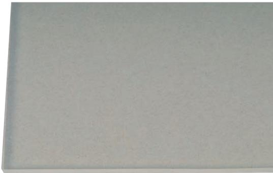
ionomer, highly break-proof, deep drawable, flexibility depending on socket wall thickness, moldable at approx. 165 °C, colour: translucent
