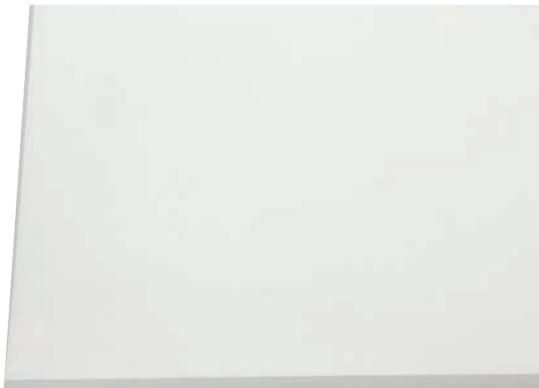
soft polyethylene, moldable at 130-160 °C, deep drawable, weldable at higher temperatures, colour: milky-white
