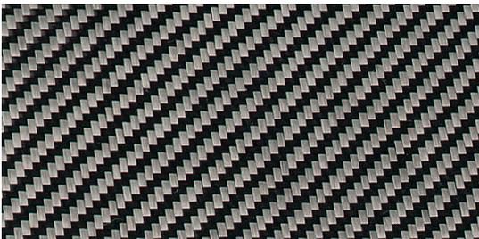
for very rigid two-dimensional lamination reinforcements in twill weave, 250 g/m<sup>2</sup>
