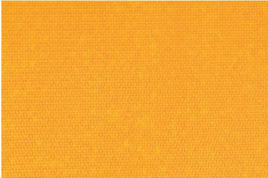
bi-directionally woven, Kevlar fiber to avoid breaking cut-outs
