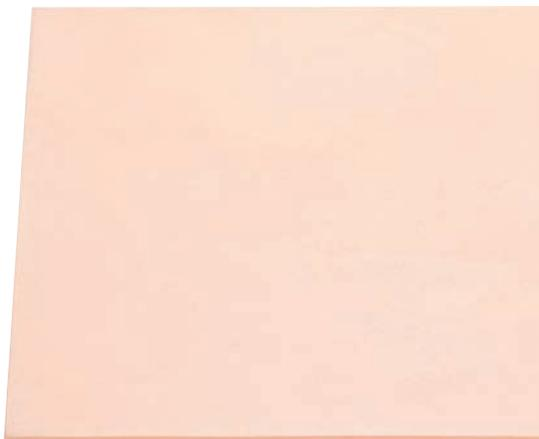
soft polyethylene, moldable at 130-160 °C, deep drawable, weldable at higher temperatures, colour: peach
