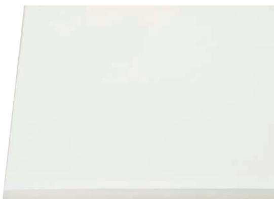
polypropylene especially designed for orthopaedic applications, moldable at 185-210 °C (e. g. in an infra-red drier) respectively at 200-210 °C (e. g. on a heating plate), weldable, deep drawable, colour: milky-white/clear-white
