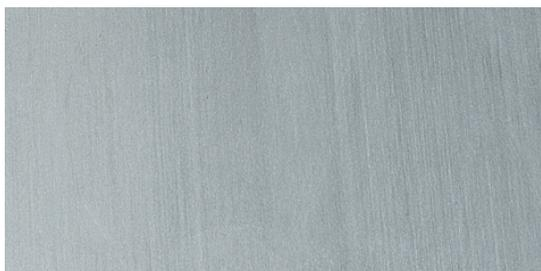
special orthopaedic quality, tensile strength 400 N/mm<sup>2</sup>, for insole supports as well as support splints of all kinds
