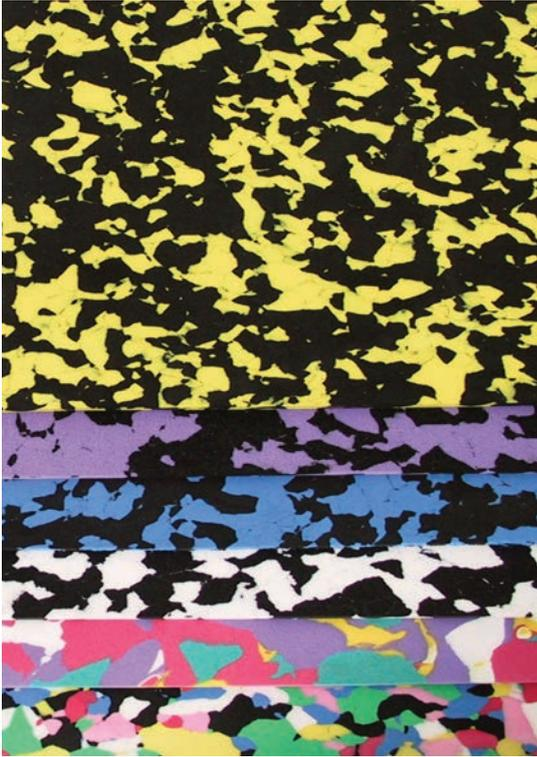
polyethylene foam, for cushionings for building ortheses as well as insoles, moldable at 130-135 °C, deep drawable, non shrinking, good restoring force
