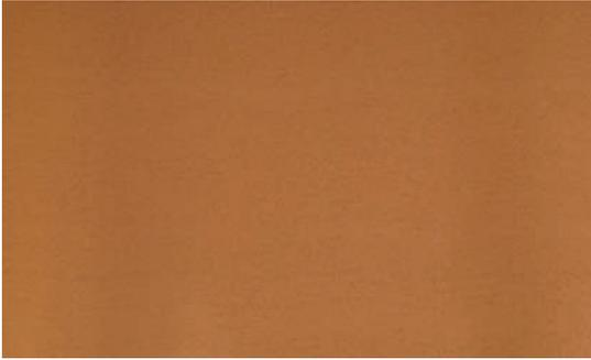
good deep-drawing abilities, this EVA-material is suitable for building insoles and supplements, at approx. 150-180 °C
